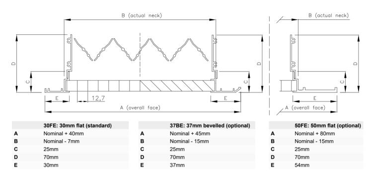
Please note: If a tile replacer size is required, for example 595mm x 595mm or 1195mm x 595mm, a 30FE 30mm flat frame should be specified.
